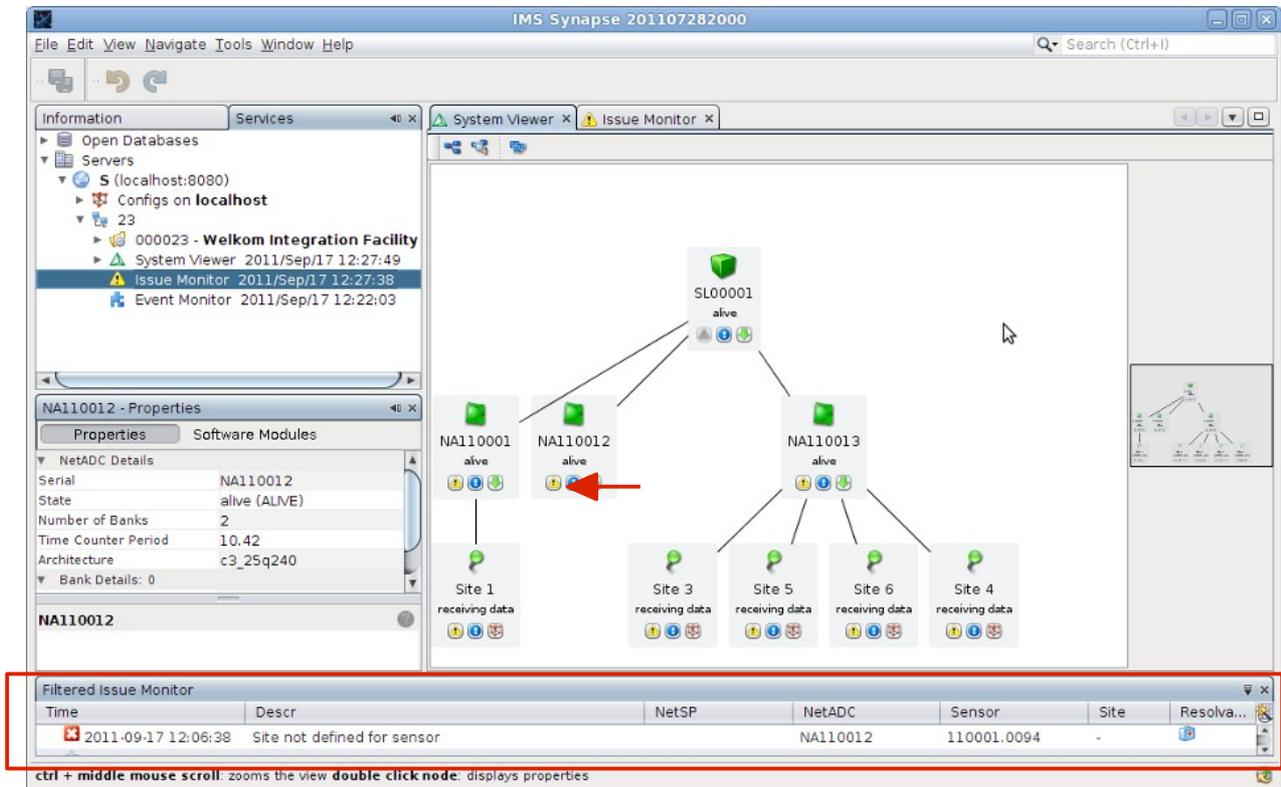
The filtered Issue Monitor reports that there is a sensor connected to the netADC that does not have a site defined.
